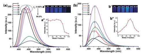
Fig. 3 Fluorescence spectra of (a) NIB and (b) NIBD at different water fractions in DMF. Insets: digital photographs of (a') NIB and (b') NIBD at different water fractions in DMF at 365 nm irradiation along with plots of  $\lambda_{emi,max}$  (a") NIB and (b") NIBD at different water fractions in DMF (10  $\mu$ M, excited at 355 nm). These experimental details validate the ACQ and AIEE characteristics of NIB and NIBD respectively.
