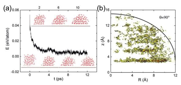
Fig. 4 (a) Temporal evolution of a water nanodroplet (containing 125 water molecules) on free-standing graphene. (b) Density contour of the nanodroplet from the last 2 ps trajectory. The solid line denotes schematically for the boundary of a spherical cap of 12 Å cap radius and 90° cap angle located 3 Å above graphene.
