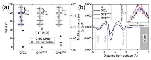
Fig. 3 Calculated for graphene on Cu (111), (chemisorbed) Ni (111) and (physisorbed) Ni (111) metal substrates: (a) •: WCA; — and ×: Mulliken charge before (dry) and after (wet) water wetting; (b) planar-averaged electron density difference and water density profile (inset).
