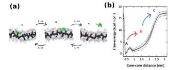
Fig. 20 (a) Snapshots of CG-BTA in water from well tempered MD representing state A, B and C, (b) free-energy profile of monomer exchange with water as a solvent.<sup>97</sup>
