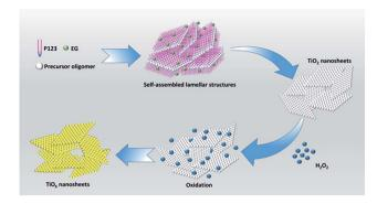
Scheme 1 Schematic representation for the synthesis of TiO<sub>x</sub> nanosheets. Here precursor oligomer is a mixture of titanium tetrachloride and hydrochloric acid.
