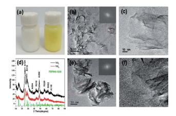
Fig. 1 (a) A photo comparing  $TiO_2$  and  $TiO_x$ . (b and c) TEM images of  $TiO_2$  nanosheets. (d) XRD patterns of  $TiO_2$  and  $TiO_x$  (A: anatase, R: rutile). (e and f) TEM image of TiOx nanosheets.
