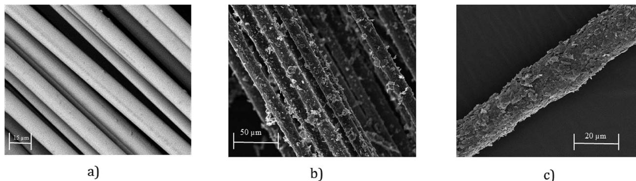
Fig. 4 (a) SEM image of untreated glass fibre roving ( $\times 2000$ ); (b) SEM image graphene-based (coated) glass roving ( $\times 500$ ); and (c) SEM image graphene-based (coated) glass roving ( $\times 1000$ ).
