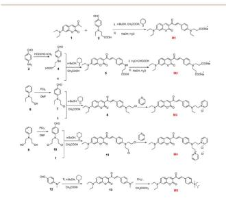
Fig. 1 Synthetic routes to targeted PSs M1-M5
