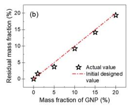
Fig. 6 (a) TGA curves of pure PTFE and GNP-PTFE nanocomposites. (b) Actual residual mass fraction of PTFE nanocomposites as a function of the initial designed mass fractions of GNP.
