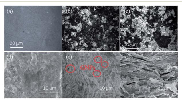
Fig. 4 Metallographic microscope images for the surface of pure PTFE (a), 10% GNP-PTFE nanocomposite (b) and 20% GNP-PTFE nanocomposite (c). SEM images for the surface of pure PTFE (d), 10% GNP-PTFE nanocomposite (e) and 20% GNP-PTFE nanocomposite (f).
