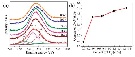
Fig. 5 (a) High resolution O1s spectra of the un-doped graphene (G) and boron-doped graphene samples (BGs) and (b) the relationship between the content of the graphitic  $sp^2$  B species (BC<sub>3</sub>) and ketone carbonyl groups (C=O) over different samples.
