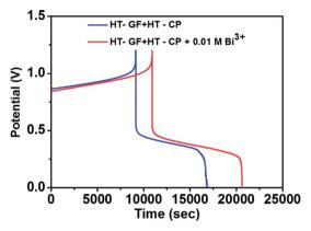
Fig. 7 Charge-discharge curves of a Fe/Cu RFB with and without  $0.01~M~Bi^{3+}$  in the electrolytes at a current density of 20 mA cm<sup>-2</sup>.
