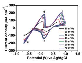
Fig. 3 CV curves of 1.8 M CuCl in a mixed supporting electrolyte (2.4 M  $CaCl_2 + 2.4$  M HCl) solution using GC electrode at various scan rates.
