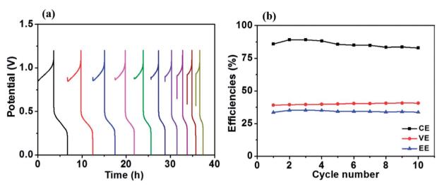
Fig. 8 (a) Charge-discharge cycling curves and (b) stability test of the Fe/Cu RFB with 0.01 M  $\rm Bi^{3+}$  at a current density of 20 mA cm<sup>-2</sup>
