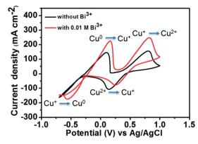
Fig. 5 CV curves of 1.8 M CuCl in a mixed supporting electrolyte (2.4 M  $CaCl_2 + 2.4$  M HCl) solution using GC electrode with and without 0.01 M  $Bi^{3+}$  at a scan rate of 50 mV  $s^{-1}$ .
