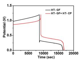
Fig. 6 Charge-discharge curves of Fe/Cu RFB cells with HT-GF and HT-GF + HT-CP at a current density of 20 mA cm $^{-2}$ .
