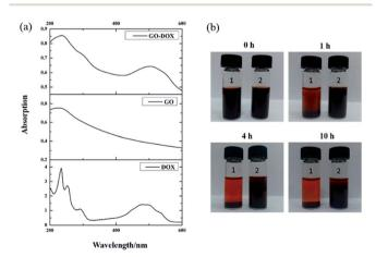
Fig. 3 The UV-vis spectra (a) of DOX, GO, and GO-DOX and the digital photos (b) for stability investigation of F127-GO-DOX hydrogel (sample 2) with GO-DOX (sample 1) solution as a control at different times
