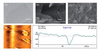
Fig. 1 (a) TEM image of GO sheets. (b) SEM image of GO sheets. (c) SEM image of F127-GO. (d) AFM image of GO.
