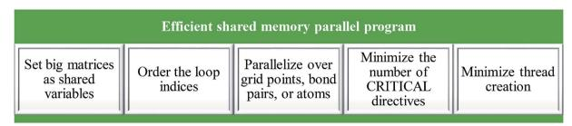
Fig. 6 Elements for achieving an efficient shared memory parallelization of the DDEC6 method.
