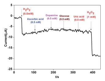
Fig. 11 The amperometric response of AgNPs-rGO-PANI-GC electrode towards H<sub>2</sub>O<sub>2</sub> and various interferential compounds (ascorbic acid, dopamine and glucose) in 0.1 M phosphate buffer (pH 7.0)
