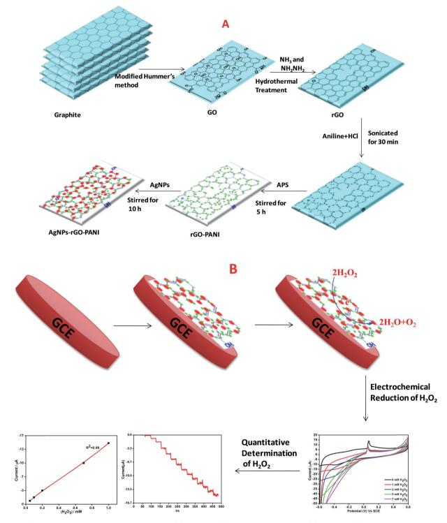
Scheme 1 Schematic representation of preparation of (A) AgNPs-rGO-PANI nanocomposite, (B) AgNPs-rGO-PANI modified glassy carbon electrode.
