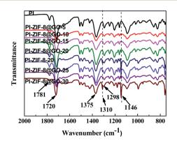
Fig. 8 FT-IR spectra recorded for the membranes.
