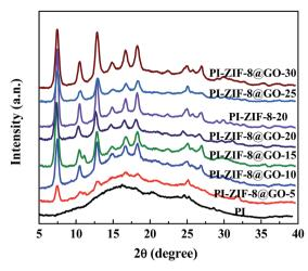
Fig. 7 XRD patterns recorded for the membranes
