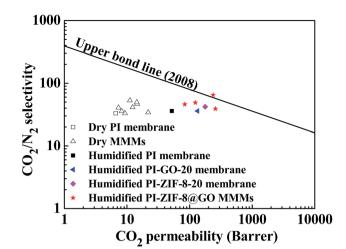
Fig. 15 Robeson's plots for CO<sub>2</sub>/N<sub>2</sub> separation
