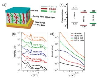
**Fig. 9** (a) An illustration for ternary OSC devices with parallel-like blends. (b) The energy level for the donor (PDBT-T1) and acceptors (ITIC-Th and PC $_{71}$ BM). (c) Out of plane (solid line) and in plane (dotted line) line cut profiles of GIWAX results of ITIC-Th:PC $_{71}$ BM blend films with different ITIC-Th contents. (d) RSoXS profiles of ITIC-Th:PC $_{71}$ BM blend films with different ITIC-Th contents. Reproduced with permission. Opportunity 2017, American Chemical Society.
