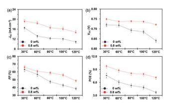
Fig. 7 Device stability of PTB7:PC<sub>71</sub>BM based OSCs without and with the PNDI2OD-T2 additive (0.8 wt%) exposed to different temperatures (30, 60, 80, 100, and 120 °C): (a)  $J_{SC}$ ; (b)  $V_{OC}$ ; (c) FF; and (d) PCE. Reproduced with permission.<sup>89</sup> Copyright 2016, Royal Society of Chemistry
