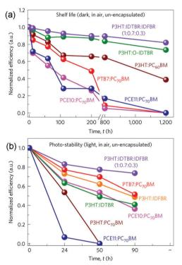
**Fig. 5** Storage lifetime (a) and photo-stability (b) tests for various blend compositions. Reproduced with permission. <sup>79</sup> Copyright 2016, Nature Publishing Group.
