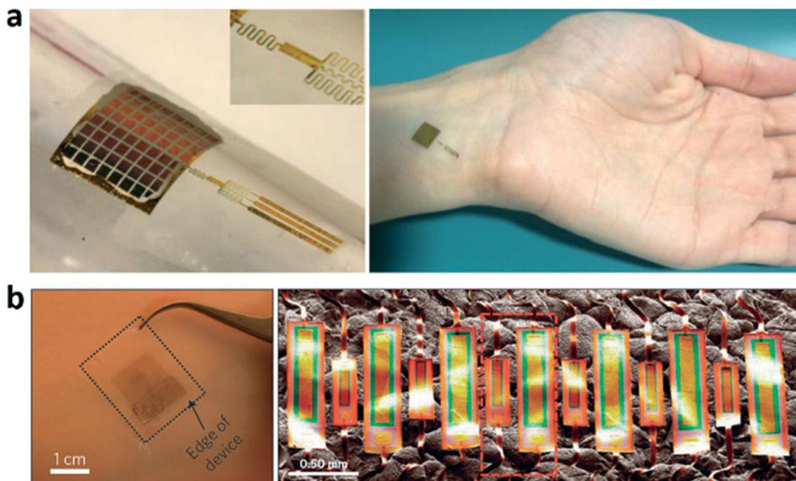
**Fig. 11** (a) Photograph of the piezoelectrical pressure sensor wrapped on a cylindrical glass support and laminated on a wrist. (b) Photographs of a piezoelectric device fully laminated on the skin and its SEM image on an artificial skin sample for tissue viscoelasticity measurement.
