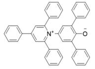
Fig. 1 Pyridinium N-phenoxide betaine, Reichardt's dye (1).
