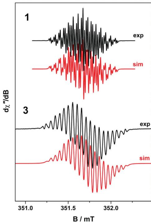
**Fig. 2** Comparison of the X-band EPR spectrum of **1** (experimental conditions: frequency, 9.8461 GHz; power, 0.63 mW; modulation, 0.007 mT), and **3** at 293 K (experimental conditions: frequency, 9.8653 GHz; power, 0.63 mW; modulation, 0.02 mT) recorded in MeCN solution at 293 K. Experimental data are represented by the black lines and simulation depicted by the red traces.
