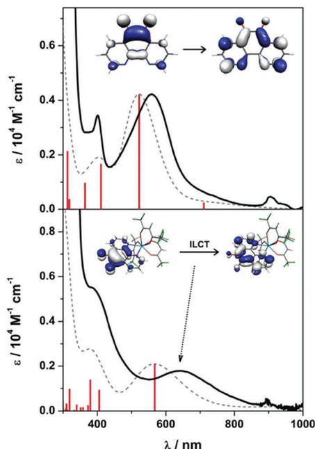
Fig. 4 Overlay of the experimental (solid line) and calculated (dashed line) electronic absorption spectra for **1** (top) and **3** (bottom) recorded at ambient temperature in MeCN. Vertical bars represent individual calculated transitions. Inset orbitals depict the donor/acceptor molecular orbitals (MO) that constitute the band at 558 nm in **1** and 639 nm in **3**.
