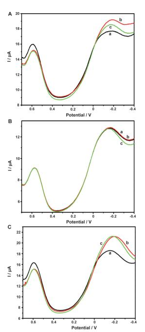
Fig. 4 DPV curves obtained on ABTS-PDDA/CNTs-NKB-GC toward 1.8 (red curve, b) and 3.8  $\mu$ g mL<sup>-1</sup> A $\beta_{1-42}$  (green curve, c) in the presence (A) and absence (B) of 6.0  $\mu$ M Cu<sup>2+</sup> PBS buffer. (C) The DPV responses of 10  $\mu$ L NaOH additions (b and c) to 6.0  $\mu$ M Cu<sup>2+</sup> PBS buffer.
