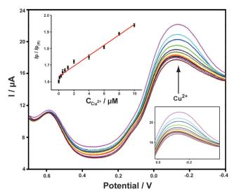
Fig. 3 DPV curves of the ABTS-PDDA/CNTs-NKB-GC toward successive additions of Cu<sup>2+</sup> at the concentrations of 0, 0.1, 0.3, 0.5, 0.8, 1.2, 2.0, 4.0, 6.0, 8.0, and 10.0  $\mu$ M. The inset is the corresponding linear plot of the  $I_P/I_{P(R)}$  ratios versus the absolute concentrations of Cu<sup>2+</sup>
