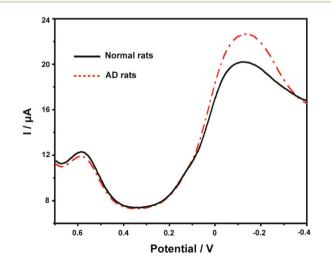
Fig. 6 DPV responses of the ABTS-PDDA/CNTs-NKB-GC on Cu<sup>2+</sup> in the plasma of normal and AD rats.
