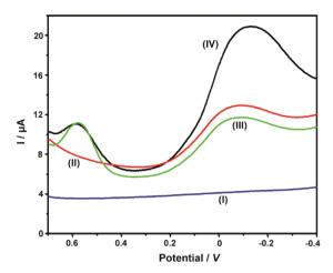
Fig. 2 DPV curves obtained on bare GC (I), PDDA/CNTs-GC (II), ABTS-PDDA/CNTs-GC (III) and ABTS-PDDA/CNTs-NKB-GC (IV) in the 100 mM PBS buffer solution containing 8.0  $\mu$ M Cu<sup>2+</sup>.
