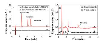
**Fig. 6** Chromatograms of the spiked sample before and after MDSPE (a) and real water sample after MDSPE (b).
