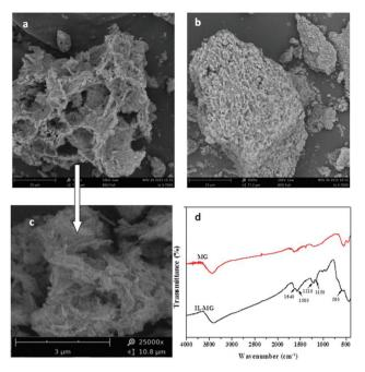
Fig. 3 Scanning electron micrograph of IL-MG (a, c), MG (b) (a: x3500; b: x3500; c: x25 000) and FT-IR spectra of MG and IL-MG (d).
