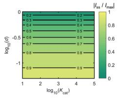
Fig. 4 Normalized steady-state current (defined as the current at T = 0.25) as a function of d and  $K_{\rm cat}$  for the enzyme-microdisc system.
