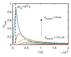
Fig. 5 Collection of the normalised current–time response to a single enzyme at a series of enzyme positions. The dashed line shows the random walk step length  $\Delta t_{\rm rw}=10^{-6}$  s. The enzyme positions  $d_{\rm enzyme}$  shown in the figure range from 5 nm to 1.5  $\mu$ m.  $r_{\rm el}=0.5~\mu$ m,  $D_{\rm P}=10^{-9}~{\rm m}^2~{\rm s}^{-1}$ .
