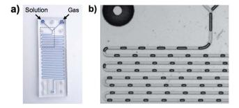
Fig. 1 (a) Schematic depiction of the MF gas/liquid device. (b) Magnified view of the outlined region shown in (a), which shows the shrinkage of the gas plugs as they flow through the channel.
