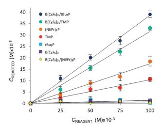
Fig. 3 Variation in equilibrium concentration of  $CO_2$  ( $C_{reacted}$ ) plotted as a function of initial reagent concentration at T=293 K (repeated in triplicate, analysing 300 images with a range of 4000-7000 plugs of  $CO_2$ ).
