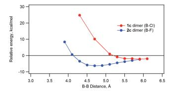
Fig. 9 Plot of the relative energy of dimeric 1c or 2c against the B–B distance calculated by *ab initio* B3LYP/6-31G(D).
