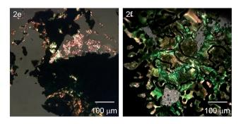
Fig. 6  $\,$  POM microphotographs of 2e and 2f at 180  $^{\circ}\text{C}$  under crossed-Nicols conditions.
