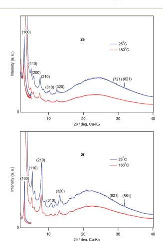
Fig. 8 Variable-temperature XRD of 2e and 2f.
