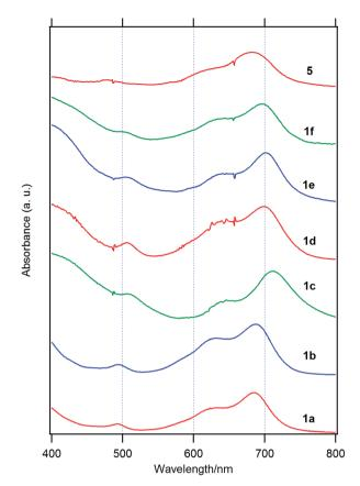
Fig. 2 Visible spectra of 1a, 1b, 1c, 1d, 1e, and 1f and the parent chloroboron(III) subnaphthalocyanine 5 on silicate glass.
