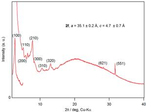
Fig. 7 Powder X-ray diffraction patterns of 2d–f. Lattice constants, a and c, were determined by least-squares fitting based on the hexagonal lattice:  $\frac{1}{d} = \sqrt{\frac{4}{3} \, \frac{h^2 + hk + k^2}{a^2} + \frac{l^2}{c^2}}$ . While the XRD patterns were recorded with a 1D silicon strip detector for a wide angle region,  $2\theta > 3^\circ$ , they were recorded with a 0D detector for the low angle region,  $2\theta = 2-5^\circ$ .
