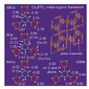
Fig. 19 Computed DDEC6 SBOs, bond orders, NACs, and ASMs for the  $\text{Cu}_3\text{BTC}_2$  metal—organic framework. Yellow lines mark the unit cell boundaries. Atoms are colored by element: H (white), C (gray), O (red), and Cu (copper). The illustrated SBOs, BOs, NACs, and ASMs are for the fully periodic crystal structure.
