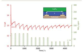
Fig. 6 Response of a 5/LuPc<sub>2</sub> MSDI heterojunction to ammonia (NH<sub>3</sub>, 90, 60 and 30 ppm), at 30% relative humidity, during exposure/recovery cycles (1 min/4 min).
