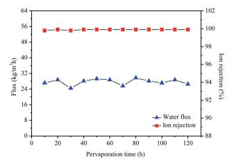
Fig. 8 Stability measurement of the GO/PI MMMs for desalination of 3.5 wt% seawater by pervaporation at  $75 \,^{\circ}\text{C}$ .
