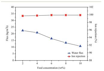
Fig. 7 Water flux and ion rejection of the GO/PI MMMs as a function of the feed concentration for desalination of different concentration seawater by pervaporation.
