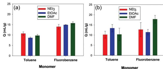
Fig. 2 Comparison of the swellingability ( $Q$ ) for toluene and fluorobenzene derived HCPs (prepared using 2 equivalents of FDA) against the three simulants triethylamine ( $\text{NEt}_3$ ), ethyl acetate (EtOAc), and dimethylformamide (DMF) using (a) Method 1 and (b) Method 2.
