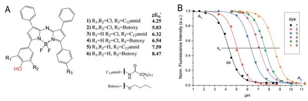
Fig. 8 A) Chemical structures of NIR emitting aza-BODIPY dyes. The protonated/deprotonated group is marked in red. Synthetic modification  $R_1$ ,  $R_2$  and  $R_3$  are used to tune the pKa value of the dyes. The lipophilic chain  $(R_3)$  is used to immobilise the dye in hydrogel polymer. B) Calibration curves of dye 1–6, embedded in a hydrogelmatrix from emission spectra. (Adapted from Strobl *et al.* 2015) reproduced from ref. 81 under the terms of the Creative Commons Attribution License.
