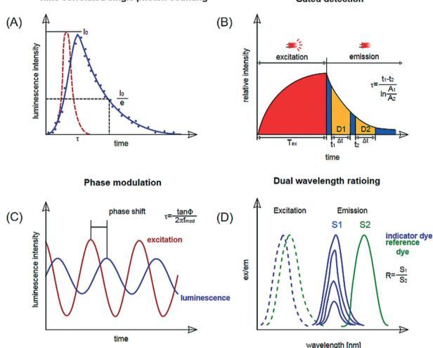
Fig. 4 Schematic representation of measurement methods applied *via* optical sensing (intensity measurements not shown). (a) Luminescence lifetime determination by time-correlated single photon counting (TCSPC). (b) Lifetime determination by gated detection: rapid lifetime determination shown. (c) Lifetime determination by phase modulation. (d) Dual wavelength ratioing. Reproduced from ref. 66 with permission from Elsevier.
