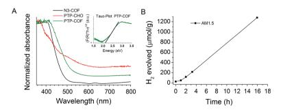
Fig. 7 (A) UV-Vis diffuse reflectance spectra of PTP-CHO and PTP-COF; (B) hydrogen evolution under AM1.5 conditions. After an initial activation period of about an hour, a linear increase in hydrogen evolution is seen.
