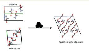
Fig. 1 Reaction scheme for the mechano-cocrystallisation of  $\alpha$ Gly + Mal to form glycinium semi-malonate.
