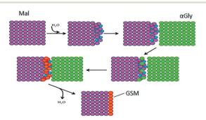
Fig. 8 Model of stepwise interactions in  $\alpha$ Gly + Mal + H<sub>2</sub>O system. Water is first sorbed by Mal, fluidising its surface. Subsequent fluidisation of the  $\alpha$ Gly surface follows, and recrystallisation of GSM
