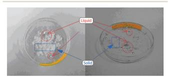
Fig. 2 Mixture of  $\alpha$ Gly and Mal at high levels of relative humidity. Liquid solution of Mal (red circles) with remaining solid powder of  $\alpha$ Gly (blue rectangles).
