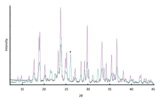
Fig. 9 Powder patterns for 1:1 mixtures of Gly: Mal loaded in ambient (green) atmosphere and dry (purple) atmosphere. The peak at 26° (marked with \*) is unique to the salt product, GSM, and it is clear that this product is formed only in the presence of a moist atmosphere.
