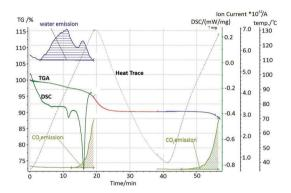
Fig. 6 Combined TGA and DSC analysis of  $\alpha$ Gly + Mal mixture after 2 hours at room level of RH (60%). The DSC and TGA traces are shown, as labelled, alongside inset mass spectrometry analysis (CO2 and water emission; ion current) for the mass loss at each stage of heating. The heat trace (dotted line) is shown as an overlay. The initial stage shows two endothermic peaks and mass loss, water and CO<sub>2</sub> emission. second stage shows only CO2 emission.
