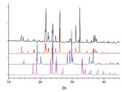
Fig. 3 XRPD pattern of the Gly + Mal mixture following "dissolution" at 100% RH, and recrystallising under ambient atmosphere (ca. 20% RH). The experimental XRPD (black) is shown alongside the simulated patterns for GSM (red),  $\alpha$ Gly (blue) and Mal (pink).
