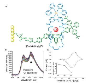
Fig. 17 (a) Surface appended electrochemical anion sensor [Os(34)(bipy)<sub>2</sub>] with bound chloride anion and (b) its optical and (c) electrochemical response to Cl.50 Adapted with permission from ref. 50. Copyright 2013 WILEY-VCH Verlag GmbH & Co. KGaA, Weinheim.
