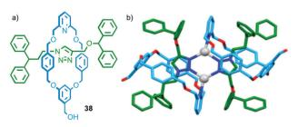
Fig. 20 (a) Interlocked rotaxane ligands 38 and (b) the solid state structure of the corresponding dimer formed in the presence of Agl. 56
