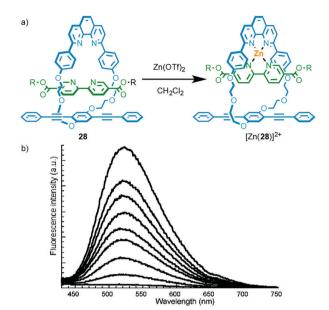
Fig. 11 (a) Emissive rotaxane 28; (b) the response of 28 to  $Zn^{II}$ . Adapted with permission from ref. 33a. Copyright 2001 American Chemical Society.
