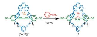
Fig. 6 Double hydroamination of rotaxane 16 mediated by an endotopically coordinationed Cul ion.21
