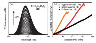
Fig. 5 (a) Steady-state PL of 3b in the presence of dodecanethiol (DDT). Increasing the amount of thiol leads to a concomitant increase in Mn<sup>2+</sup> PL from the NCs. (b) Scatter plot of the Mn<sup>2+</sup> PL intensity vs. [DDT] for NC samples with different degrees of branching. The more branched 3b NCs show the steepest increase in PL intensity with thiol. NCs with less (2) and no (6) branching show decreasing sensitivity to thiol, with smaller increases in slope.
