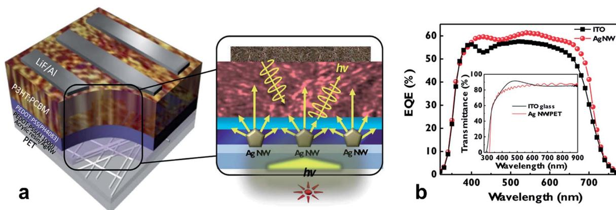
Fig. 6 (a) Schematic illustration of light scattering and trapping phenomena induced by the AgNW mesh in the device; (b) external quantum efficiency (EQE) spectra of a P3HT:PCBM OSC with the AgNW mesh electrode and the reference device with ITO; the inset depicts transmittance spectra of corresponding electrodes (reproduced with permission. Copyright 2015, Wiley VCH Weinheim).<sup>95</sup>
