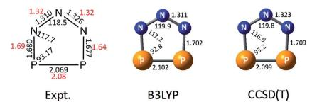
Fig. 2 Comparison of the X-ray structure of  $P_2N_3^-$  in [Na-kryptofix-221][ $P_2N_3$ ] salt (major component in black, minor component in red)<sup>27</sup> with the calculated structures at B3LYP/aug-cc-pVTZ and CCSD(T)/aug-cc-pVTZ levels of theory. Bond distances are in angstroms (Å) and bond angles are in degrees (°).
