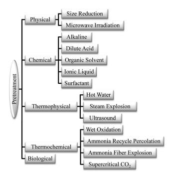
Fig. 2 Various pretreatments for lignocellulosic biomass.
