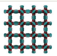
Fig. 2 Computer visualization of the ideal IRMOF-1 structure. 2 × 2 × 2 unit cells are shown under periodic boundary conditions. Cyan colour corresponds to the organic linkers, red colour indicates oxygen atoms associated with the zinc-containing vertices of the structure.
