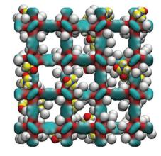
Fig. 9 On the left: computer visualization of the IRMOF-1 structure loaded with 24 molecules of DMF. On the right: the same structure shown together with the adsorbed argon molecules. Colour scheme: in IRMOF-1 cyan is for carbon, red for oxygen, grey for argon; for DMF, nitrogen is blue, carbon is yellow, oxygen is red and hydrogen is grey.
