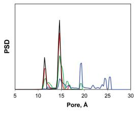
Fig. 4 On the left: accessible surface area ( $m^2 q^{-1}$ ) in IRMOF-1 as a function of the percentage of linkers removed. Line is for eye guidance only. On the right: geometric pore size distribution as a function of the percentage of linkers removed. Black line is for 0% (perfect crystal), red line is for 50%, green line is for 65% and blue line is for 73% linkers removed.
