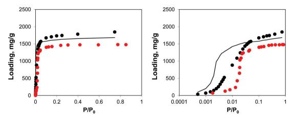
Fig. 10 Adsorption isotherms for argon at 78 K in IRMOF-1. Red symbols are the experimental results, 7.26 black symbols are from molecular simulations, black line corresponds to the system with residual DMF. The panel on the right uses the logarithmic pressure scale.
