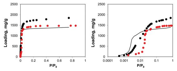
Fig. 12 Adsorption isotherms for argon at 78 K. Red symbols are the experimental results, 7.26 black symbols are from molecular simulations, black line corresponds to the system loaded with gold nanoclusters. The panel on the right uses the logarithmic pressure scale.
