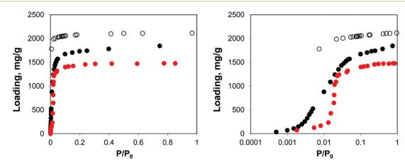
Fig. 3 Adsorption isotherms for argon at 78 K in IRMOF-1. Red symbols are the experimental results, 7.26 open symbols are unscaled simulation results from Dubbeldam and co-workers, 26 black symbols are from molecular simulations in this work. The panel on the right uses the logarithmic
