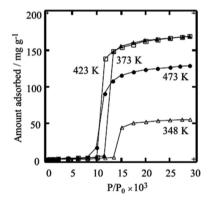
Fig. 16 Gate opening behaviour for CO<sub>2</sub> adsorption in a Cu(II) MOF. Reprinted with permission from ref. 56, Copyright (2001) Elsevier.
