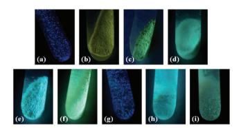
Fig. 25 Naked eye fluorescence changes in a guest responsive dynamic MOF upon immersion in several volatile organic solvents (a) parent compound, (b) acetonitrile, (c) methanol, (d) ethanol, (e) tetrahydrofuran, (f) benzene, (g) cyclohexane, (h) cyclohexane (longer time), (i) dichloromethane. Reproduced from ref. 76, Copyright (2013) The Royal Society of Chemistry.
