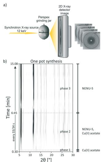
Fig. 3 a) Schematic representation of the setup used for the *in situ* investigations of the mechanochemical syntheses of NENU-5. b) 2D plot of synchrotron XRD data for the mechanochemical one pot synthesis (reaction 4) of NENU-5 with a description of the detected compounds; Cu(ii) acetate = copper(ii) acetate monohydrate.
