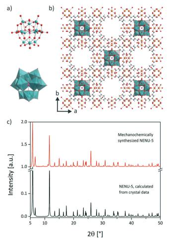
Fig. 1 a) Structure of the Keggin-type POM [PMo<sub>12</sub>O<sub>40</sub>]<sup>6-</sup> shown as ball-and-stick and polyhedra model. b) Structure of NENU-5 consisting of empty pores and pores filled with Keggin ions (polyhedra). Orange: copper, turquoise: molybdenum, pink: phosphorus, red: oxygen, grey: carbon, light grey: hydrogen. c) Comparison of the diffraction pattern of the mechanochemically synthesised NENU-5 with the calculated diffraction pattern.
