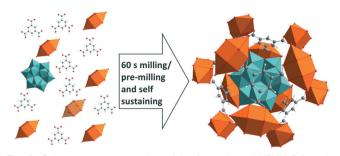
**Fig. 4** Schematic representation of the formation of NENU-5 from its building units. Orange polyhedra:  $Cu_2O$ -cluster, turquoise polyhedron:  $[PMo_{12}O_{40}]^{6^-}$ , ball-and-stick representation: 1,3,5-benzenetricarboxylic acid with red: oxygen, grey: carbon, light grey: hydrogen.
