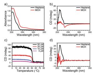
Fig. 2 (a) UV-Vis absorption of **2** in heptane and MCH in a high concentration regime (7.5 mM, 20 °C); (b) CD spectra of **2** in heptane and MCH in a high concentration regime (7.5 mM, 20 °C); (c) TD-CD of **2** in heptane ( $\lambda_{max}$  = 211 nm, concentration range 50–5  $\mu$ M, cooling speed 50 °C h<sup>-1</sup>); (d) CD spectra of **2** in heptane and MCH in a low concentration regime (20  $\mu$ M, 20 °C).
