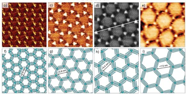
Fig. 3 Isoreticular host networks based on van der Waals interactions between alkyl chains. (a) Molecular structure of the DBA derivatives. STM images of honeycomb porous networks formed by (b) DBA-OC10 (c) DBA-OC14, (d) DBA-OC20 and (e) DBA-OC30. Panels (f-i) show molecular models for the corresponding porous networks, respectively. Reproduced from ref. 54, 53 and 40 with permission from the American Chemical Society, Wiley-VCH and the Royal Society of Chemistry, respectively.
