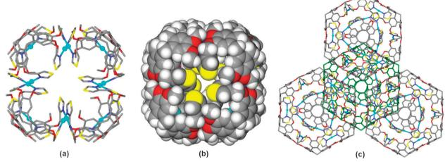
Fig. 2 From the crystal structure of  $[Aq_{12}(L)_8] \cdot 12ReO_4 \cdot n(DMF)$  **1** showing (a) the  $[Aq_{12}(L)_8]^{12+}$  cube; (b) space-filling view; (c) partial packing of cubes through  $\pi - \pi$  stacking interactions into a cubic close packed array.
