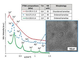
Fig. 3 SAXS profiles of PTBA films with varying thymine—adenine ratio or varying nucleobase block weight percent; TEM image shows ordered lamellar morphology of a PTBA (9.4–20.0–3.4) triblock copolymer film. \*Newton's rings are imaging artifacts due to weak phase contrast.
