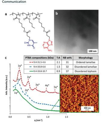
Fig. 1 (a) Chemical structure of poly(ThA-b-nBA-b-AdA) (PTBA) ABC triblock copolymers. (b) TEM image of the PTBA (9.4-31.5-4.6) triblock copolymer film. (c) SAXS profiles of PTBA films with varying thymineadenine molar ratio; AFM phase image shows the disordered biphasic surface morphology of a PTBA (9.4-33.8-10.7) triblock copolymer film.
