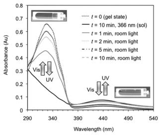
Fig. 4 Reversible changes in the UV/Vis spectra for an organogel in toluene showing the reversible trans-to-cis isomerisation of the azobenzene moiety. On irradiation with UV light, the trans isomer changes to the cis isomer, leading to a gel-to-sol transition. Reproduced from ref. 47 with permission from the Royal Society of Chemistry.
