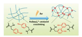
Fig. 19 Irradiation of a tyrosine-containing LMWG in the presence of a ruthenium catalyst leads to cross-linking and a dramatic increase in gel strength. Reproduced from ref. 135 with permission of the Royal Society of
