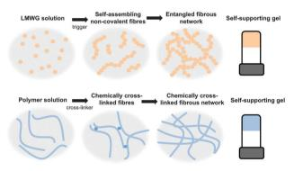
Fig. 1 Gelation using (top) low molecular weight gelators, where the crosslinks are generally formed by entanglement and (bottom) polymers, where the cross-links can be permanent chemical bonds or entanglements
