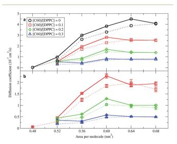
Fig. 7 Diffusion coefficients of (a) DPPC lipids and (b) fullerenes as a function of the area per molecule. The systems consisted of 400 (dot line) and 1600 (solid line) molecules per monolayer. The error bars for DPPC are of the size of the symbols. Diffusion coefficients were not calculated in simulations with an area per molecule of 0.48 nm<sup>2</sup> and  $[C_{60}]/[DPPC]$  ratios of 0.2 and 0.3 because the monolayers collapsed.
