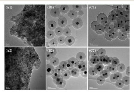
Fig. 11 TEM images of  $Pd_{imp}/SiO_2$  (A),  $Pd_{cub}@SiO_2$  (B) and  $Pd_{pol}@SiO_2$  (C) catalysts before (1) and after (2) catalytic test. Reproduced from ref. 128 Copyright (2015), with permission from Elsevier.
