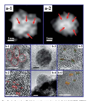
Fig. 5 (a-1 and a-2) High-angle annular dark field (HAADF) STEM images of Ni nanoparticles in Ni/H–Al $_2$ O $_3$ . (b-1–b-6) HRTEM images of Ni nanoparticles selected from the Ni/H–Al $_2$ O $_3$  sample (the scale bar is 2 nm). Reprinted with permission from ref. 52 Copyright (2013) American Chemical Society.
