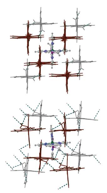
Fig. 5 Packing diagrams of 1[ClO<sub>4</sub>]<sub>2</sub> in phase 1 at 253 K (top) and phase 2 at 240 K (bottom). The pale coloured cations are in the same layer as the highlighted molecule, whereas the dark cations are in adjacent layers to the front and back. The close intermolecular  $C-H\cdots\pi$  contacts involving the methylsulfanyl groups are also indicated (tabulated in the ESI†).
