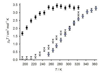
Fig. 6 Variable temperature magnetic susceptibility data for 1[BF<sub>4</sub>]<sub>2</sub> in  $(CD_3)_2CO$  ( $\bullet$ ),  $2[BF_4]_2$  in  $(CD_3)_2CO$  ( $\triangle$ ) and  $3[BF_4]_2$  in  $CD_3NO_2$  ( $\bullet$ ).
