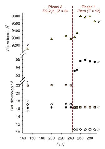
Fig. 3 Temperature dependence of the crystallographic unit cell dimensions, and the unit cell volume normalised to Z = 12, for  $1[ClO_4]_2$ . The dashed line indicates the crystallographic transition temperature.
