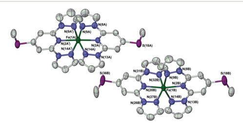
Fig. 4 View of the two crystallographically unique [Fe(L<sup>SMe</sup>)<sub>2</sub>]<sup>2+</sup> cations in phase 1 of 1[ClO<sub>4</sub>]<sub>2</sub> at 280 K. Atomic displacement ellipsoids are at the 50% probability level, and H atoms have been omitted for clarity. The atom numbering scheme in phase 2 is the same as for molecule B of phase 1 (ESI†). Symmetry code: (i) 1 - x, y, 3/2 - z. Colour code: C, white; Fe, green; N, blue; S, purple.
