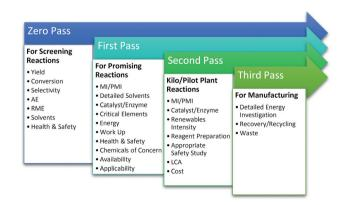
Fig. 2 Structure of the metrics toolkit showing the parameters covered
