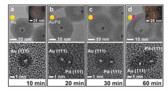
Fig. 2 TEM (upper) and HRTEM (lower) images of samples isolated during the reaction of the  $(Fe_3O_4/Au)@(SiO_2/Pd^{2+})$  with NaBH<sub>4</sub> at (a) 10, (b) 20, (c) 30, and (d) 60 min, respectively. Insets: EDX elementary maps for showing the distribution of Au (red) and Pd (yellow) elements.
