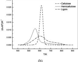
Fig. 1  $\,$  Experimental TG and DTG curves of cellulose, hemicellulose and lignin.
