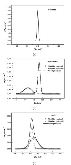
Fig. 6 The f(E) curves estimated for cellulose, hemicellulose and lignin.
