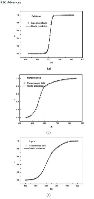
Fig. 5 Experimental and calculated  $\alpha(T)$  curves of cellulose, hemicellulose and lignin by integrating the calculated DTG curve.
