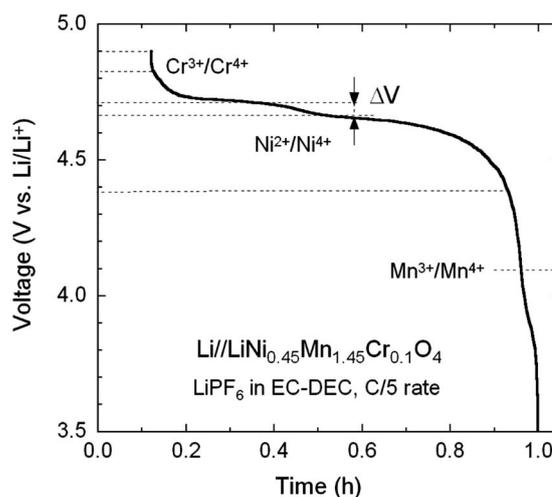
Fig. 8 Typical voltage profile of charge of a Li//Cr-doped LNM cell showing the various redox reactions  $\text{Mn}^{3+/4+}$  (at 4.1 V),  $\text{Ni}^{2+/4+}$  (at 4.7 V) and  $\text{Cr}^{3+/4+}$  (at 4.8 V).
