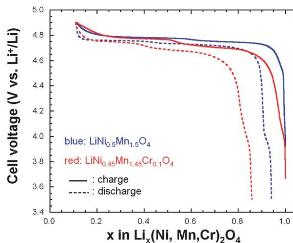
Fig. 10 Charge–discharge curves of the un-doped and Cr-doped LNM cathodes in CR2032 coin cell composed of  $\text{LiPF}_6$  in EC–DEC (1 : 1) as electrolyte. The cathode electrode contained 89 wt% active material, 6 wt% conductive carbon, and 5 wt% PVdF binder (loading  $5 \text{ mg cm}^{-2}$ ). All cells were cycled at 25 °C between 3.5 and 4.9 V at C/5 rate.
