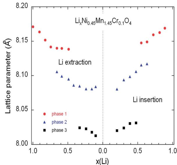
Fig. 14 Variation of the lattice parameters of the different cubic phases in the Cr-doped LNM sample as a function of the Li concentration  $x$  during the charge (a) and discharge (b) during cycling at  $C/24$  rate. Reproduced with permission.<sup>77</sup>
