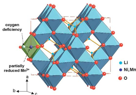
**Fig. 1** The structure of spinel  $\text{LiNi}_{0.5}\text{Mn}_{1.5}\text{O}_4$  ( $Fd\bar{3}m$  S.G.). Oxygen deficiency partially reduces  $\text{Mn}^{4+}$  to  $\text{Mn}^{3+}$  to satisfy local charge neutrality.
