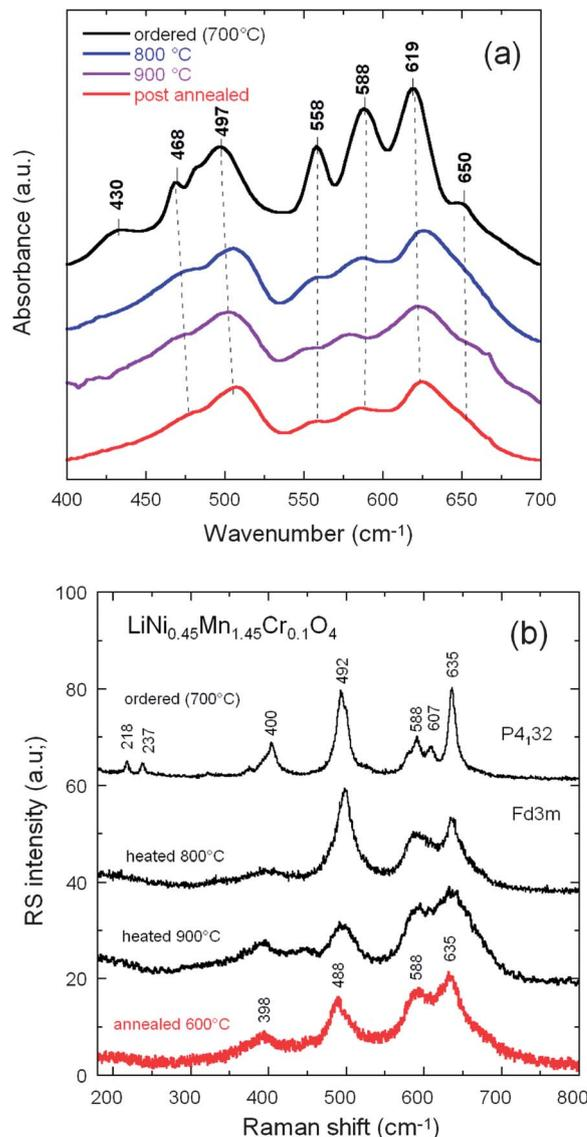
Fig. 5 FTIR (a) and Raman scattering (b) spectra of the  $\text{LiNi}_{0.45}\text{Mn}_{1.45}\text{Cr}_{0.1}\text{O}_4$  samples obtained at different steps of the synthesis: at different temperatures up to 900 °C before annealing, and for the final sample, post-annealed at 600 °C for 48 h.
