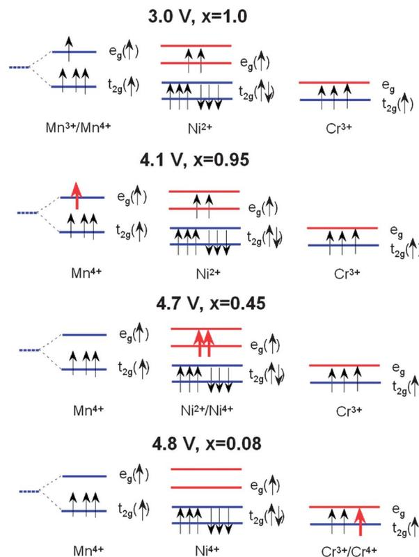
Fig. 9 Schematic diagram showing the 3d electronic levels of  $\text{Mn}^{3+}$ ,  $\text{Ni}^{2+}$  and  $\text{Cr}^{3+}$  in  $\text{LiNi}_{0.5-y}\text{Mn}_{1.5-y}\text{Cr}_{2y}\text{O}_4$  spinel during the charge process. It is noted that  $\text{Ni}^{2+}$  favours the low-spin configuration in  $\text{LiNi}_{0.5-y}\text{Mn}_{1.5-y}\text{Cr}_{2y}\text{O}_4$ . Partially empty levels are shown with red arrows.
