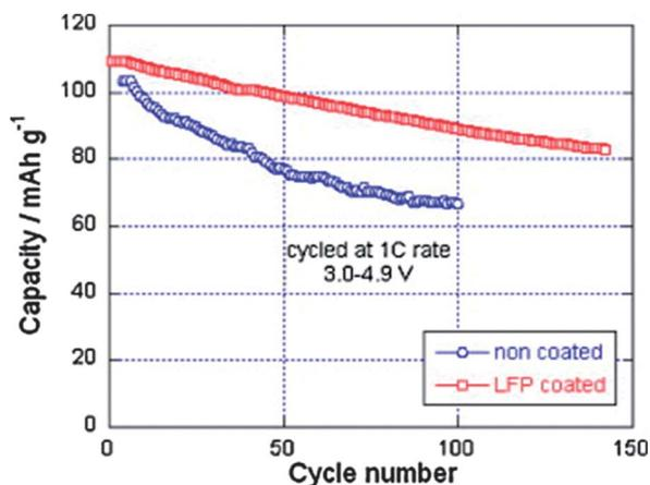
Fig. 17 Cyclability of the Li//LMN and Li//LFP-coated LMN cells at 1 C between 3.0 and 4.9 V vs. Li<sup>+</sup>/Li<sup>0</sup>. Reproduced with permission.<sup>86</sup>
