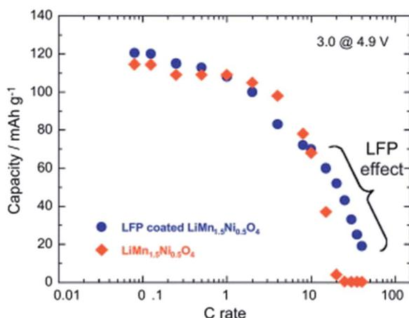
Fig. 16 Modified Peukert plot for the Li//LMN and Li//LFP-coated LMN cells between 3.0 and 4.9 V vs. Li<sup>+</sup>/Li<sup>0</sup>.
