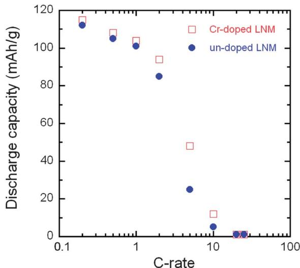
Fig. 12 Modified Peukert curves of LNM and  $\text{LiNi}_{0.45}\text{Mn}_{1.45}\text{Cr}_{0.1}\text{O}_4$  spinel cathodes cycled between 3.5 and 4.9 V in CR2032 coin cell with  $\text{LiPF}_6$  in EC–DEC (1 : 1) as electrolyte.
