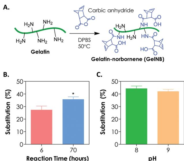
**Fig. 1** (A) Schematic of gelatin-norbornene (GelNB) synthesis. (B) Effect of reaction time (without pH adjustment) on the degree of norbornene substitution (\**p* < 0.05). (C) Effect of the solution pH value on the degree of norbornene substitution. In all reactions, carbic anhydride was added at 20 wt/vol%.
